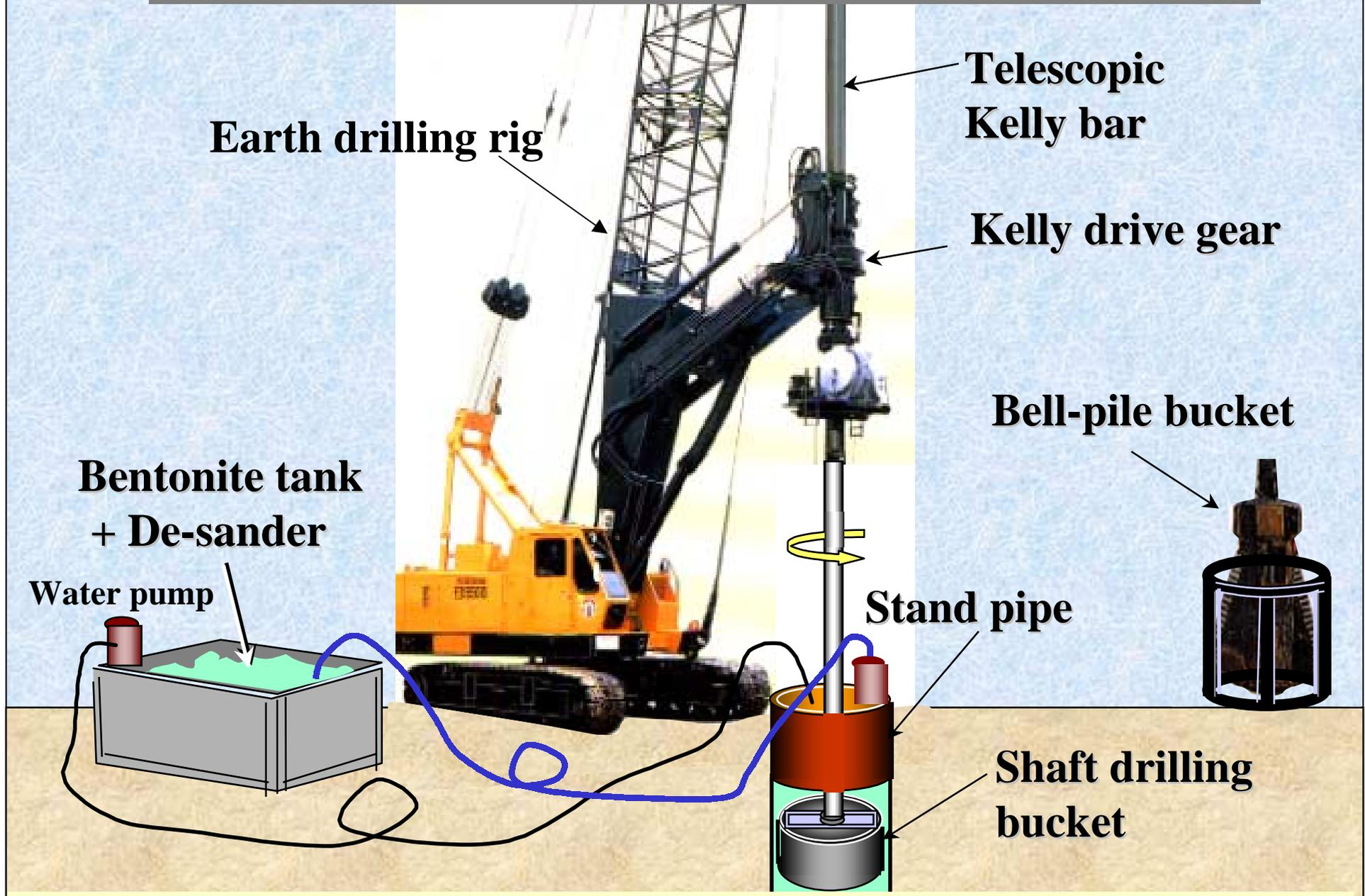
Necessary equipment for [Bell-pile technique] consist of an earth drilling rig equipped with Kelly drive + Kelly bar, shaft drilling bucket ( + Bell-pile bucket, stand pipe, water pumps + hoses, Bentonite mixer/ de-sander / tank. After drilling the bore hole shaft to the specified depth, replace the shaft drilling bucket with bell-pile bucket to ream the bottom area of the bore hole.
