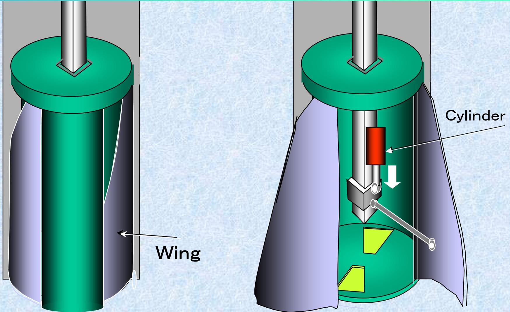
A pair of wings are opened and closed through a sliding rod by a pair of cylinders. An opening ratio of the wing can be detected with a sensor in the cylinder.
