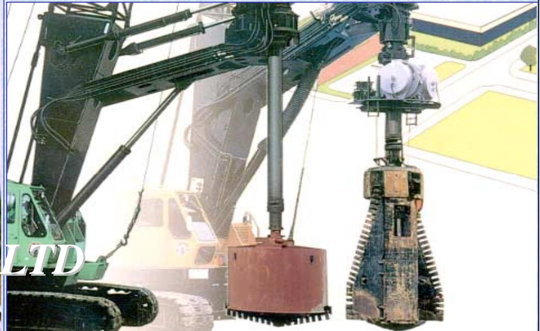
This [Bell pile technique] which is able to increase the end-bearing capacity of the pile by enlarging its bottom sectional area, has come into wide use in Japan This chapter summarizes outline, work process and equipment of [Bell pile technique] by the use of NISSHA ED-series earth drilling rigs equipped with telescopic Kelly bars and BK-series bell buckets.
