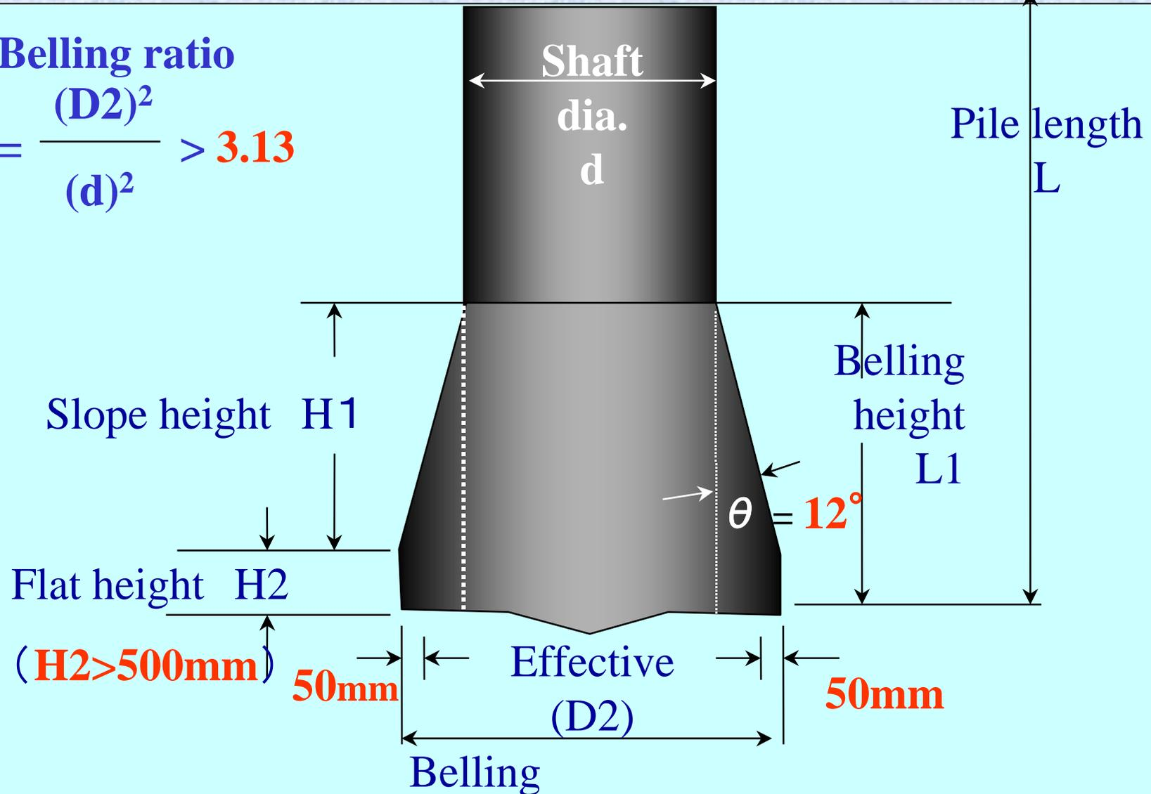
Dimensions of belling out are detailed by Ministry of Construction in Japan as shown above. The effective belling out diameter of the bell-pile is actual belling diameter  $D1$  minus  $100\text{mm}$  ( $50 + 50$ ).
