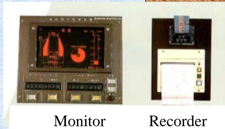
The opening ratio of the belling bucket is detected electrically by the cylinder and its electrical data is transmitted through a radio transmitter to the receiver on the earth drill rig. Bell-pile construction data are monitored and recorded through a monitor and a recorder in the operator's cabin.
