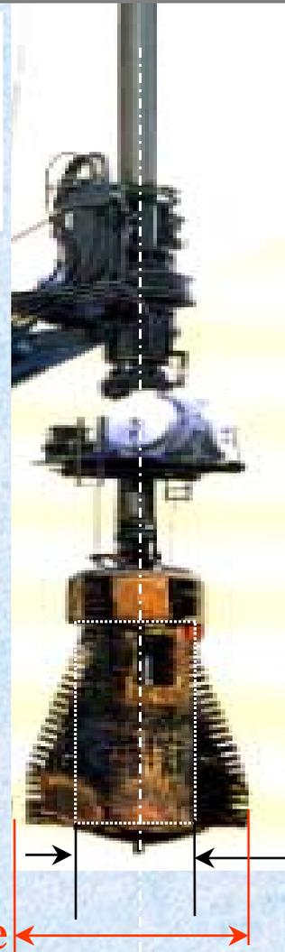
Comparison between [Straight pile] and [Bell-pile], if the shaft diameter is the same, then the end bearing area of the bell-pile is twice and more than the one of straight pile. Or if the end bearing area is the same, then the concrete amount to be poured to the bell-pile is half and less than the amount of straight pile.
